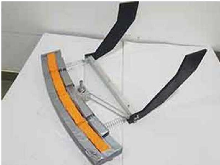
The device will prevent car from going under a truck through an energy absorbing pivoting mechanism.
