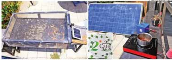
(L) Spices being baked using solar cooker; tea being made on electric stove drawing power from solar panel (R)
